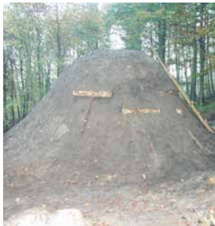
fertiger Kohlemeiler, © C. Schmit
